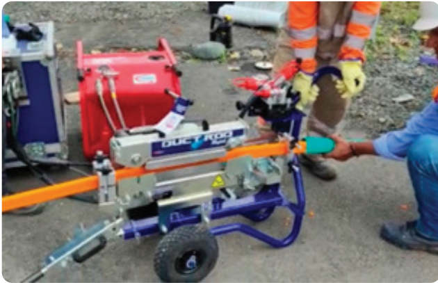
DuctRod RAPID set up with micro duct between chains.
