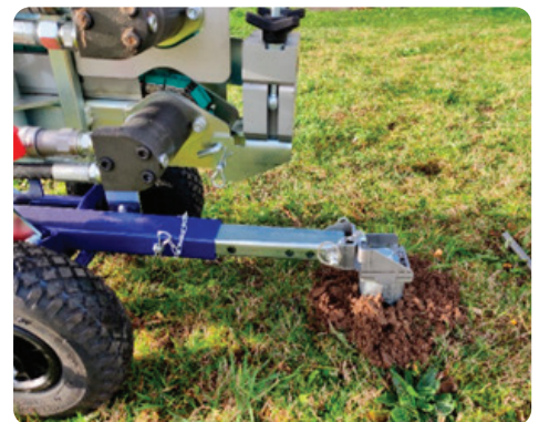
Ground Fixture fully installed with machine connected.
